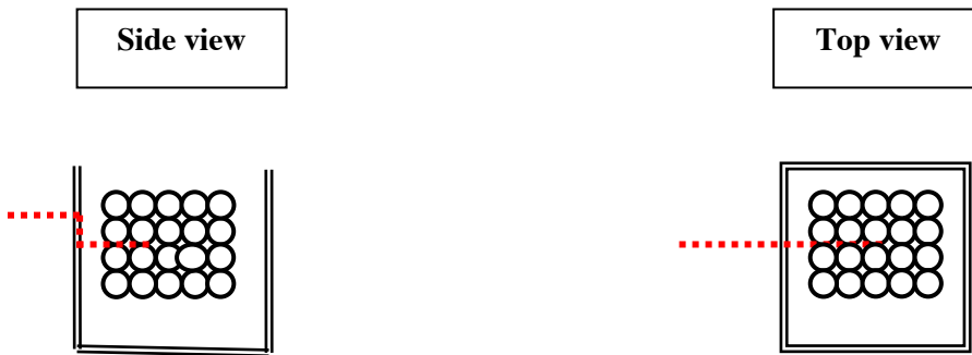
Figure 4. Styrofoam box showing placement of temperature probe (••••) from side view (A) and view from top of box (B).
