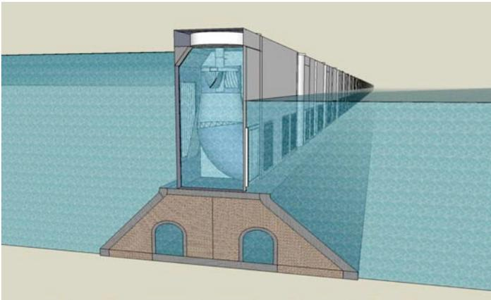
The navigation gates could contain a number of different types of turbine. Illustrated are vertical shaft turbines with conventional screens.
