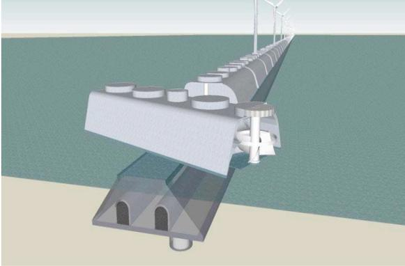
Illustrated is a rotatable group of turbines that allow unidirectional turbine operation, screen cleaning and water to bypass the 'Reef'
