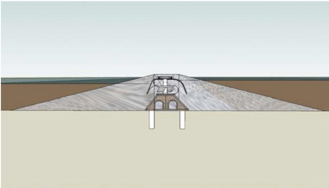
A section of the 'Reef' superimposed on the outline of a typical rock and sand embankment. The difference in material content can clearly be seen.
