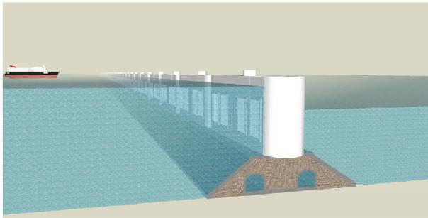
The navigation gates not only provide the access for deep draught ships but for the unimpeded flow of water when high upstream levels must be achieved.
