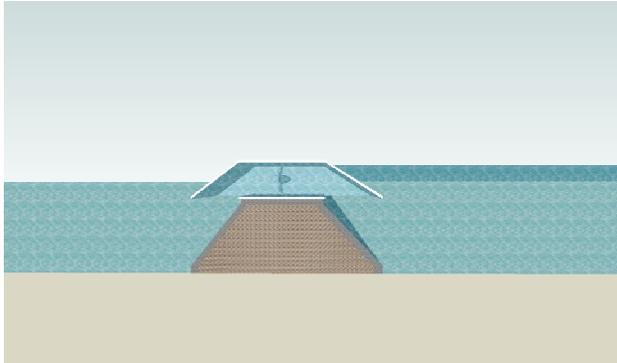
The turbine caissons could be of a horizontal duct form with 'Darrius' 'Crossflow' or 'Propeller' turbines, provided they could meet with the overall environmental criteria and in particular, being 'fish friendly'.
