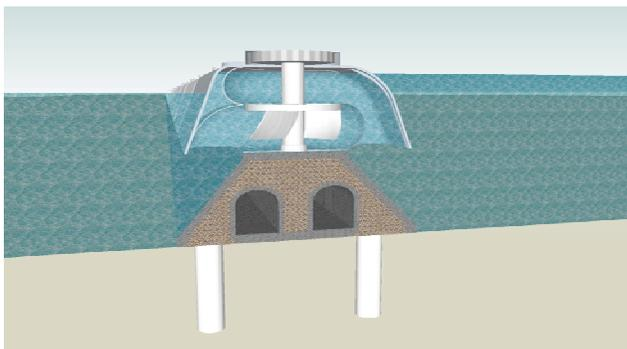
An alternative method of construction at the 'Shoots Location' might employ a 'Causeway' that included railway tunnels as part of the base structure.
