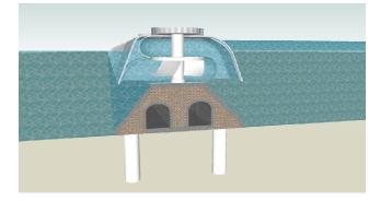
An alternative method of construction at the 'Shoots Location' might employ a 'Causeway' that included railway tunnels as part of the base structure.
