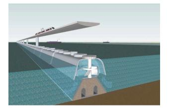
The main vertical piles of the 'Reef' structure could be extended upwards to provide support for a railway bridge, but provision would have to be made for shipping.
