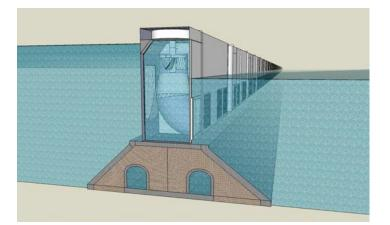
The navigation gates could contain a number of different types of turbine. Illustrated are vertical shaft turbines with conventional screens.
