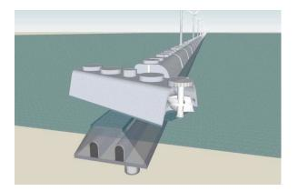
Illustrated is a rotatable group of turbines that allow unidirectional turbine operation, screen cleaning and water to bypass the 'Reef'
