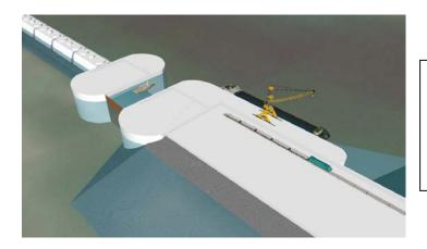
Illustrated is the transition between the rock embankment with its railway transfer sidings and a turbine section with a small boat lock in between.
