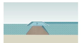
The turbine caissons could be of a horizontal duct form with 'Darrius' 'Crossflow' or 'Propeller' turbines, provided they could meet with the overall environmental criteria and in particular, being 'fish friendly'.
